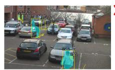
The motion object tracker is ideal for sterile environments, where only valid objects should cause events to be produced. The motion object tracker reduces the false events caused by foliage and other environmental factors and can create events for valid objects that are detected.
