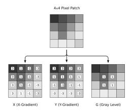
As frames are processed, the X, Y and G-values are statistically modelled using gaussian models. Each gaussian model keeps a running average of the mean and variance of the X, Y and G-values sampled from each patch i.e.  $3\times$  mean values, and  $3\times$  variance values. A sample is within the gaussian if the value is contained within the range specified by the mean and variance.
