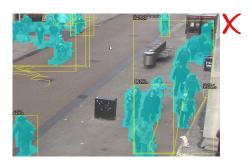
The height of the camera is also important. The lower the camera height, the larger objects will appear to the motion tracker and the more chance that objects will be bound together into a single unidentified object. It is also important to consider that the lower the camera height, the more chance of objects being obstructed by other objects in the scene.
