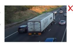
Camera positioning should avoid scenarios where objects can cross paths and merge together, for example. Cameras positioned to monitor traffic should be overhead, this minimizes object blocking.
