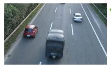
The motion object tracker will function in the scene shown in the image but vehicle movement will cause a lot of false object detection and can result in high false events. Position cameras to provide a more overhead view or look at one of the other DL trackers as an alternative solution.
